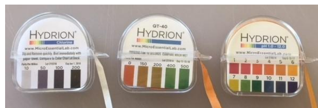
Test strips for chlorine, quat, and acid sanitizers
